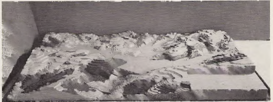
The top model shows a three dimensional model of an area scheduled for the site of a reservoir. The water level on completion of the dam was cut in blue perspex along the contour line and superimposed on the model as shown in the lower photograph. This shows in great detail and accuracy the effect of flooding on existing roads, railways, houses, farm properties, etc., and new routes for roads, railways and power lines, etc., can be easily established on the model.
