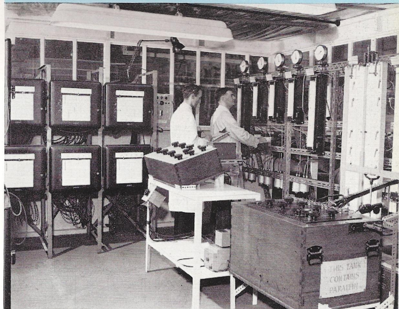
Fig. 6 (below) Part of the control and instrumentation room associated with the temperature stability test rig.
