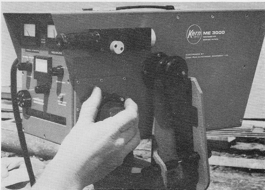
Close-up: the Kern ME 3000 Mekometer.
