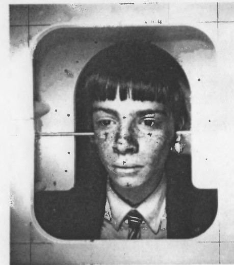
FIG. 4. Right hand view from a stereo-pair taken with the Addenbrooke's instrument showing the secondary frame in position above the datum which carries the meatal rods. Ultra-violet illumination of the subject has revealed in the skin melanin-impregnated areas which are normally invisible, resulting in a heavily freckled appearance which makes an excellent image for photogrammetric analysis.
